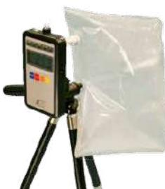
Collects samples into a sampling bag directly for air sampling in work environment.
