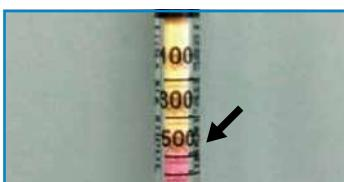
⑤ Take out the tube and read out the end point of discolouration layer to know the concentration.
