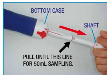
③ Align the red lines on the shaft and the bottom case and pull the handle until full to lock.
