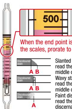
When the end point is between the scales, prorate to read out.
