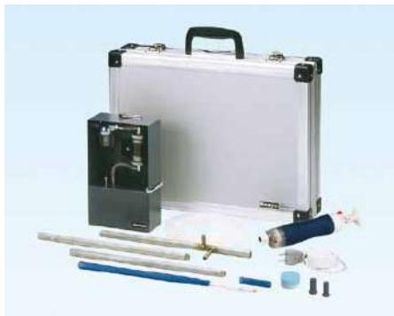
Measures gas samples from a gas duct such as Nitrogen oxides, Sulphur dioxide, Oxygen to prevent pollution easily and quickly. For voluntary control of emission standard.
